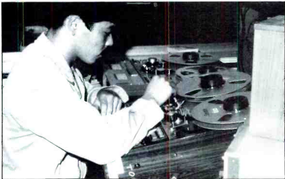
Every recording head constructed in the factory is placed in service for a complete checkout before it is released to the assembly department.
